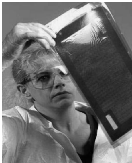
Fig. 3 Examining a large-scale, framed MEA for a 75-kW PEFC stack (courtesy of UTC Fuel Cells).
