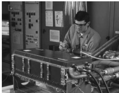
Fig. 5 A 75-kW stack under testing (courtesy of UTC Fuel Cells).
