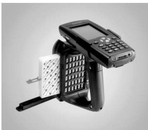
Fig. 58 Air-breathing DMFC cell array and methanol cartridge integrated into the handle of an RFID tag reader made by Intermec, Inc.
