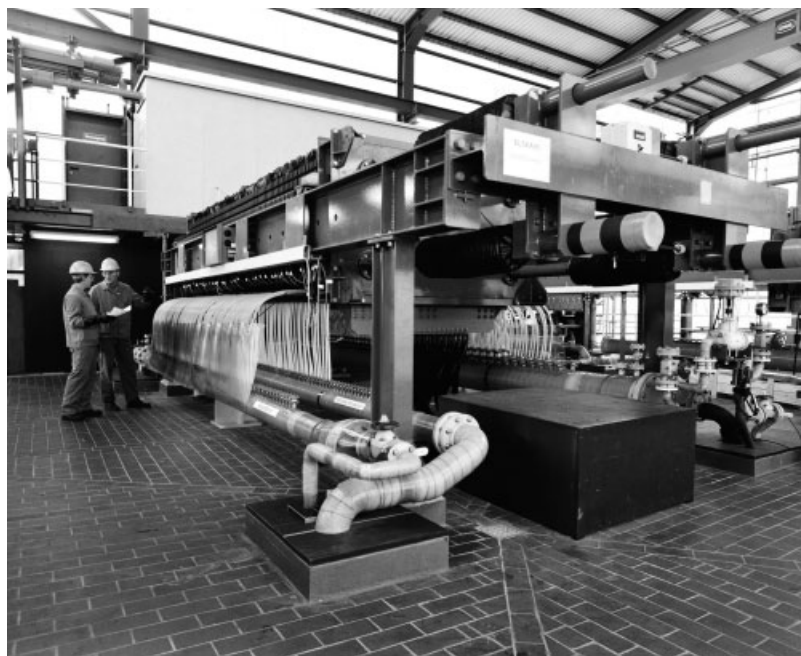
Fig. 1 Cell room of the hydrochloric acid electrolyzer with GDE in Brunsbüttel [28] (photo: Bayer Material Science AG).
