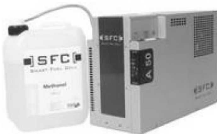
Fig. 59 A 50-W DMFC power source commercialized by Smart Fuel Cells (Germany). Volume of the 50-W (4 A; 11–14 V) stack shown is 1.3 L and it weighs 8 kg. The system efficiency is reported as 700 \text{ Wh L}^{-1} ( 0.7 \text{ Wh cm}^{-3} ) of 100% methanol stored in the tank. The system noise level is reported as low as 47 dB at a distance of 1 m.
