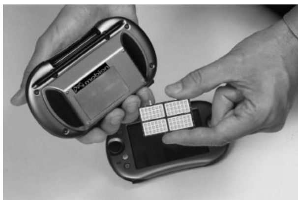
Fig. 6 The molded flat array of air-breathing DMFCs, shown held between the fingers on the right, generates power in the range 0.5–1 W in a concept prototype of a DMFC system for portable consumer electronics applications. (MTI Micro Fuel Cells).
