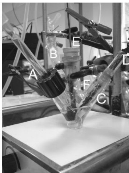
Fig. 1 View of a glass cell (capacity: 5 to 7 ml of solution) connected to a power source (potentiostat). Case of a reduction at a copper cathode. A: inlet for inert gas, B: reference electrode like a saturated calomel electrode, C: anodic compartment (a glass tube ended by a glass frit), D: platinum grid as anode, E: working electrode: copper grid (area: about 4\text{ cm}^2 ), F: inert gas outlet. The solution is stirred with a magnetic bar. Thus for an amount of electroactive compound (one-electron reduction) of 10^{-3} mol, electrolysis current could be of the order of 0.1 A and the reaction completed (until nil current) in much less than 1 hour.
