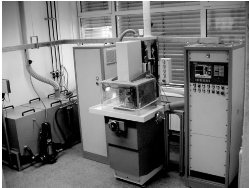
Fig. 17 ECM-1500A machine (Novotech Ltd) for electrochemical three-dimensional shaping.
