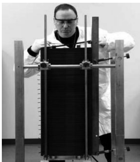
Fig. 4 Stacking the bipolar plates and MEAs for a 75-kW PEFC stack (courtesy of UTC Fuel Cells).
